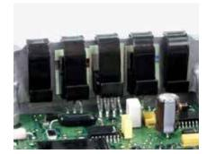
Bergquist SI-Pad A1500 is a silicone-based, thermally conductive and electrically insulating material. It consists of a cured silicone elastomeric compound coated on both sides of a fiberglass reinforcement layer.
