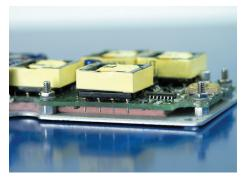
Gap Pad<sup>®</sup> VO Ultra Soft is recommended for applications that require a minimum amount of pressure on components. The viscoelastic nature of the material also gives excellent low-stress vibration dampening and shock absorbing characteristics. Gap Pad<sup>®</sup> VO Ultra Soft is an electrically isolating material, which allows its use in applications requiring isolation between heat sinks and high-voltage, bare-leaded devices.
