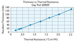
Note: Resultant thickness is defined as the final gap thickness of the application.
