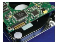
Gap Pad 2000SF is a silicone-free insulating material. Silicone-sensitive applications benefit from this fiberglass-reinforced gap filling material, which combines electrical isolation with exceptional thermal performance (2.0 W/mK). While highly thermally conductive, the material is exceptionally soft and more compliant than other silicone-free materials. Gap Pad 2000SF is capable of conforming to the most demanding contours while applying little stress on component leads.
